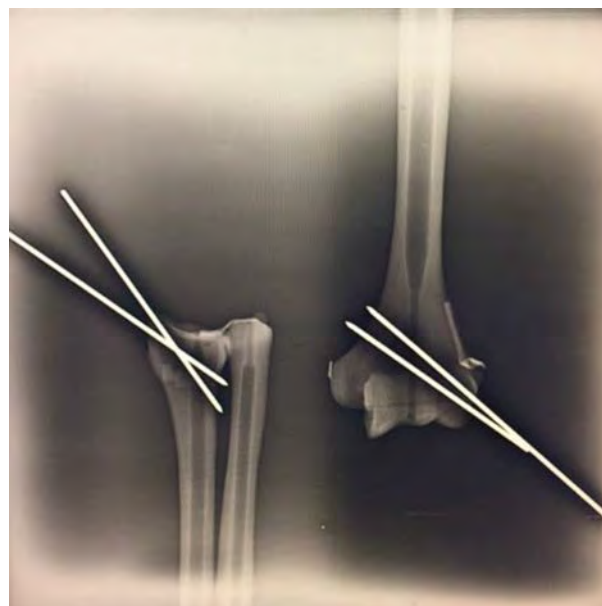
Fig. 3 Anteroposterior radiographic image of two synthetic bone models with pins placed in a manner typical for fixing supracondylar humerus and distal radius fractures.
